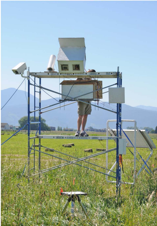
Fig. 6. (Color online) Imaging systems mounted atop 3 m tall scaffolding at the ZERT field site. The multispectral imager is behind the left window of the white instrument housing box. The tripod in the foreground holds the reflectance calibration panel
