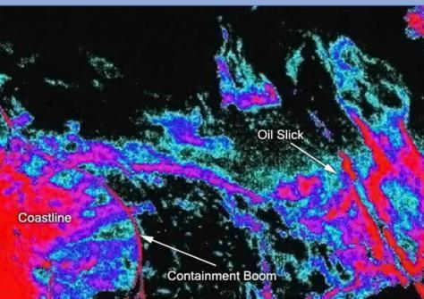
Image 2. Hyperspectral image of an oil spill
