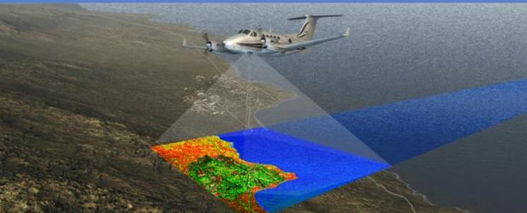
Figure 3. Aircraft equipped with digital cameras and sensors are a flexible options to obtain imagery for vegetation analysis. Aerial imagery is often incorporated in studies today due to its ability to focus on one specific location at a fine resolution. (Northrop Grumman Corporation, 2017)
