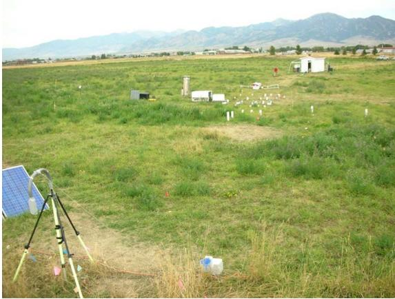
Fig. 2. Three CO<sub>2</sub> hot spots near the end of the 2009 release (long after they were detectable with multispectral imaging), along with equipment situated above the buried release pipe.
