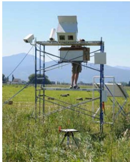
Fig. 4. Multi-spectral imager mounted along with other sensors on scaffolding at the ZERT test site. The imager views the scene through the left window (from the observer’s perspective) of the white box.
