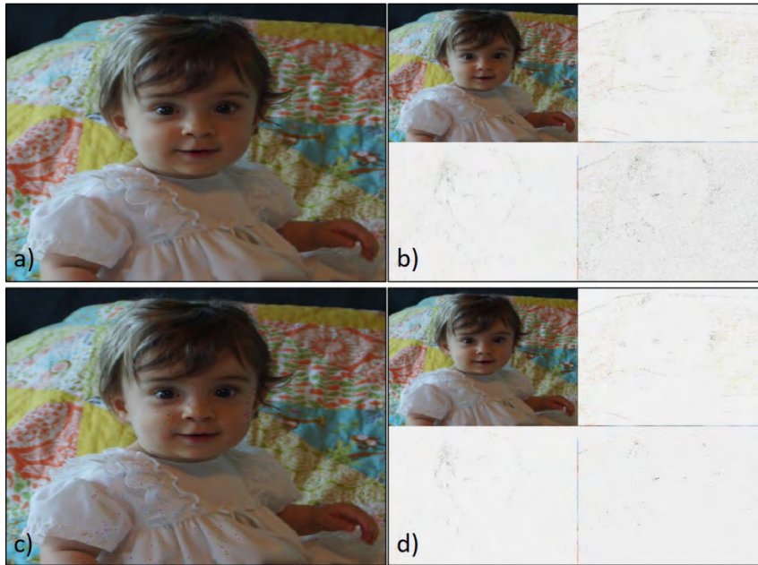
Figure 7-19. Image compression using wavelet-based image decomposition: (a) original image; (b) wavelet decomposition of original image; (c) compressed image (76.33% compression); (d) wavelet decomposition of compressed image.
