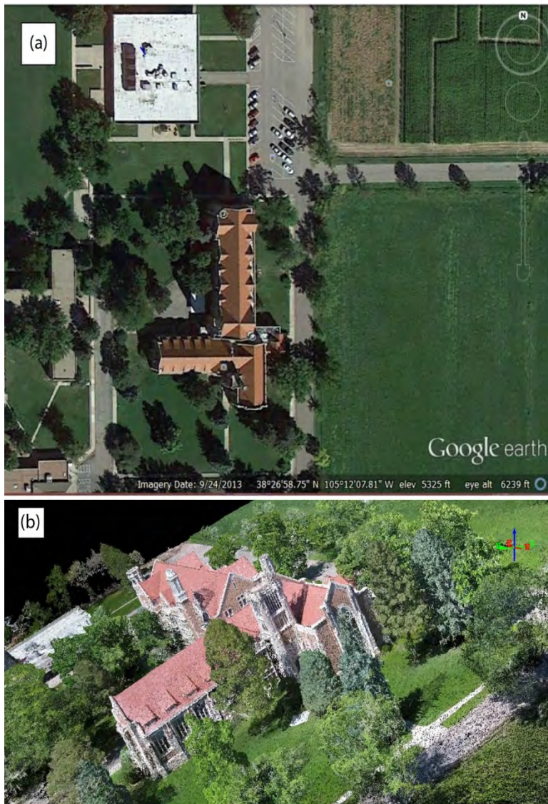
Figure 7-77. (a) Control points obtained from high resolution images are used to assign real-world coordinates to 3D models, and (b) The resulting RGB 3D point cloud.
