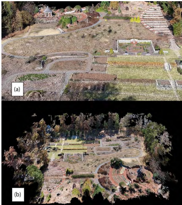
Figure 7-75 (a) 3D point cloud of the Georgia State Botanical Gardens, and (b) geovisualization of the area.
